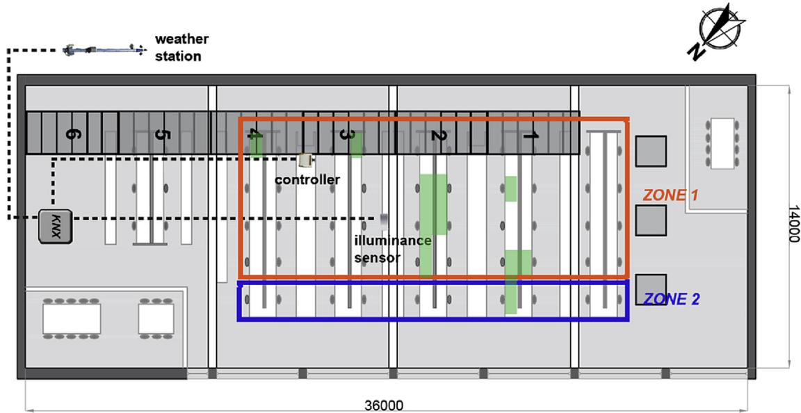
**Fig. 11.** Plan view of office space with indication of the 11 users that actuated the blinds (green coloured desks). Glare from the roof lights never occurs in zone 2 (zone in blue), for the other desks glare may occur (zone 1 in orange). (For interpretation of the references to colour in this figure legend, the reader is referred to the web version of this article.)
