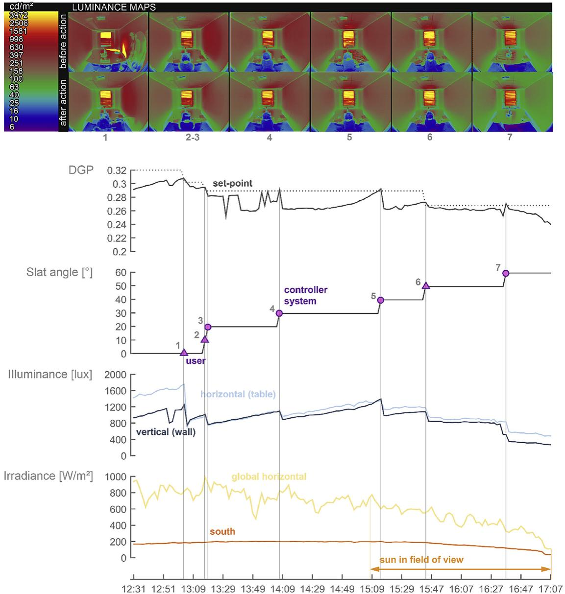
Fig. 9. The user manually overrides the control of the controller system, which results in an adaptation of the set-point.
