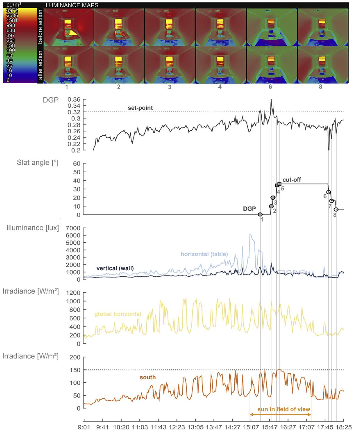
Fig. 10. The DGP control strategy is combined with the cut-off angle strategy to improve the visual comfort.
