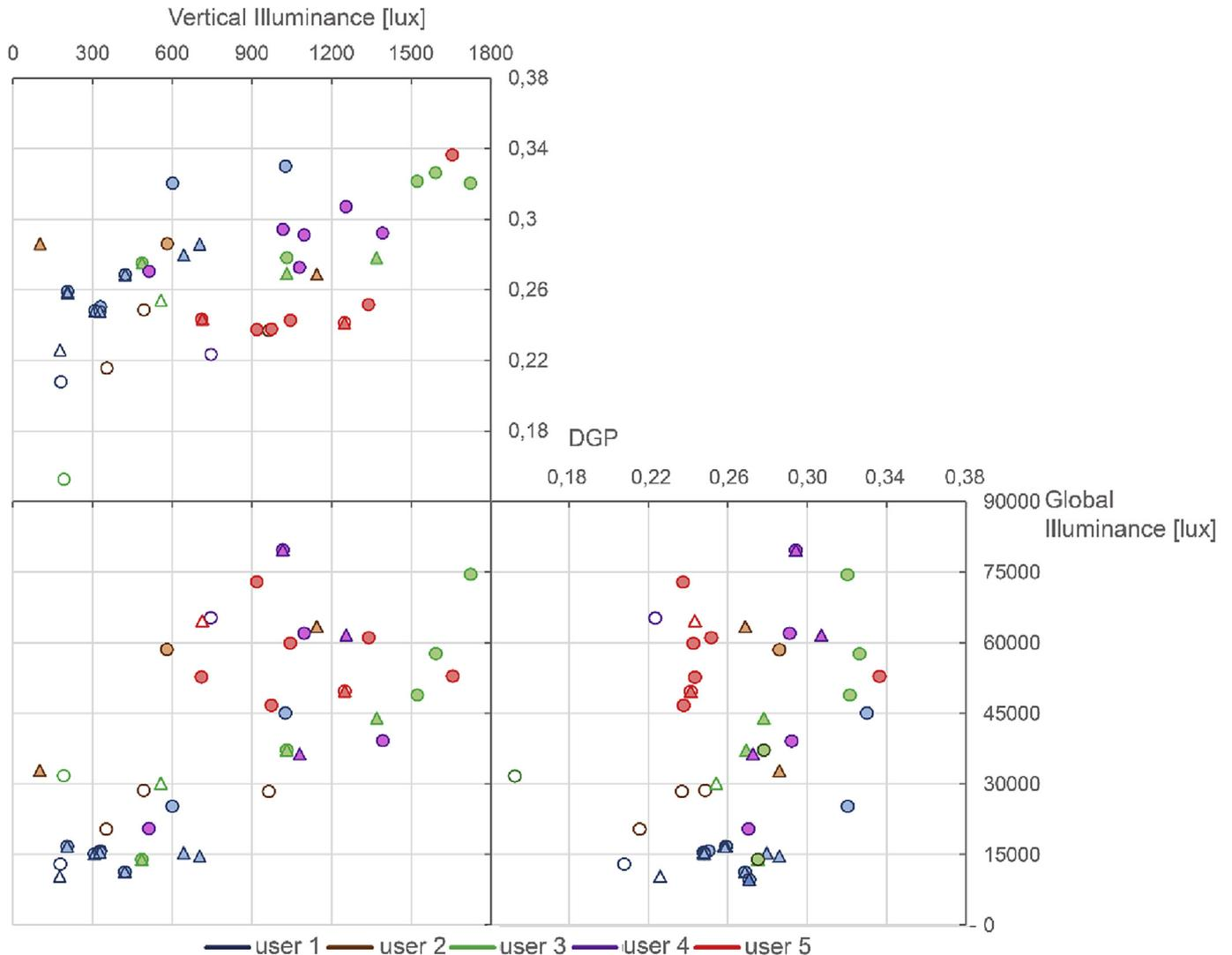
Fig. 8. Overview of the actions of the controller system (circle) or user (triangle) to put the shading system in a more closed (filled) or more open (not filled) position. The values of the DGP, vertical illuminance and global illuminance are shown on the time of the action, thus before any change to the state of the shading system occurs.
