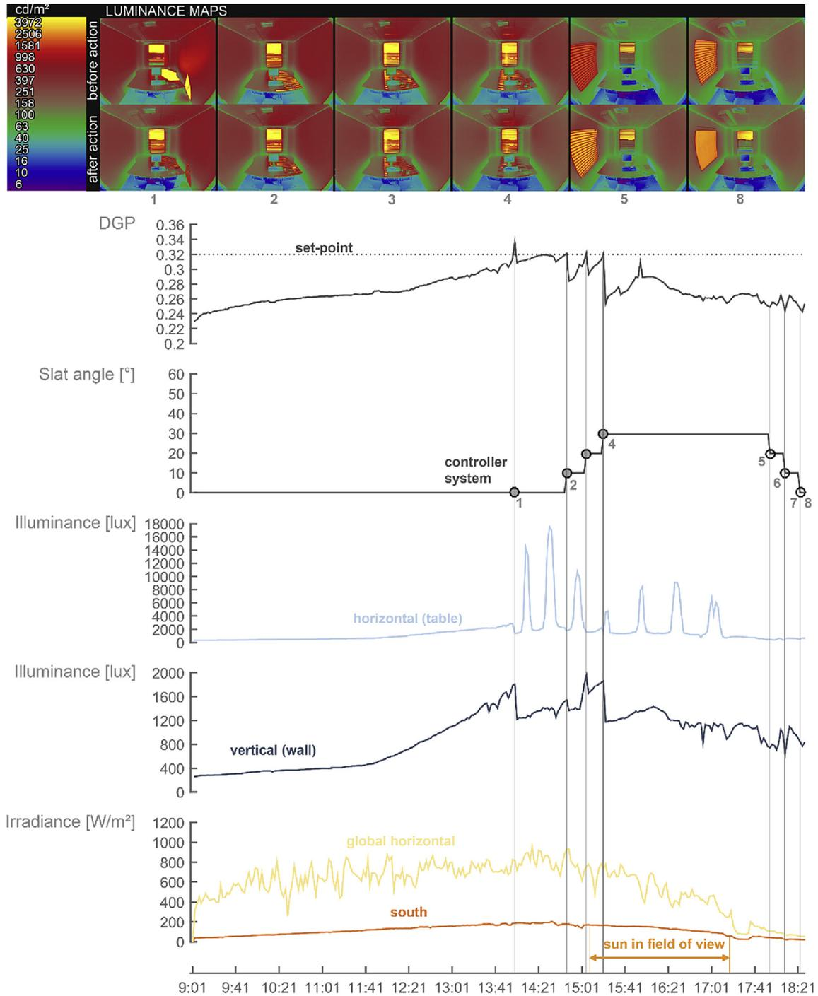
Fig. 6. The luminance maps before and after an action show how the position of the venetian blind is altered according to the predefined set-point for a sunny day in March.
