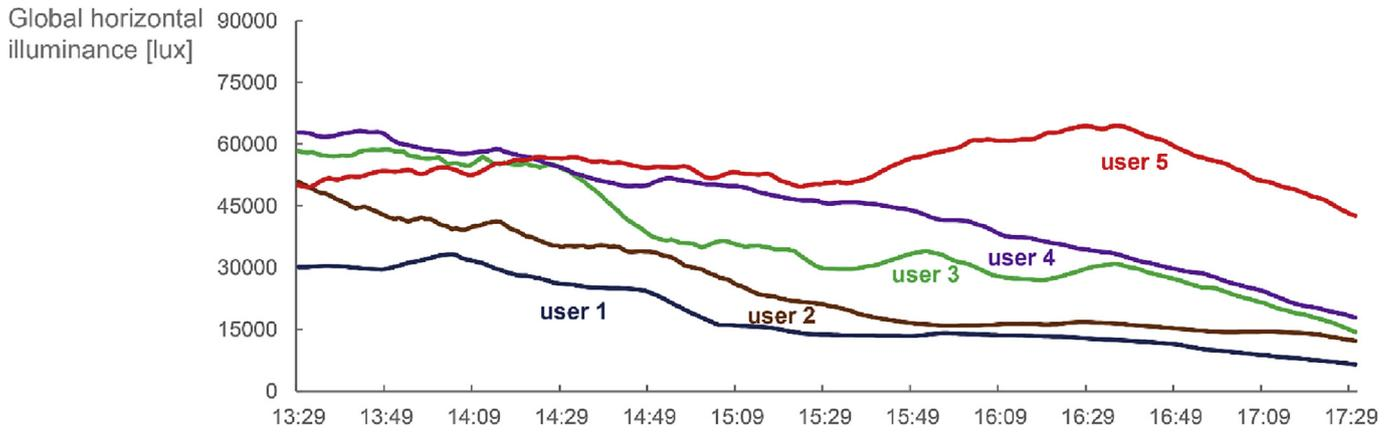
Fig. 7. A running mean graph of the global horizontal illuminance outside during the different measurements with the users shows the varying weather conditions during the test.
