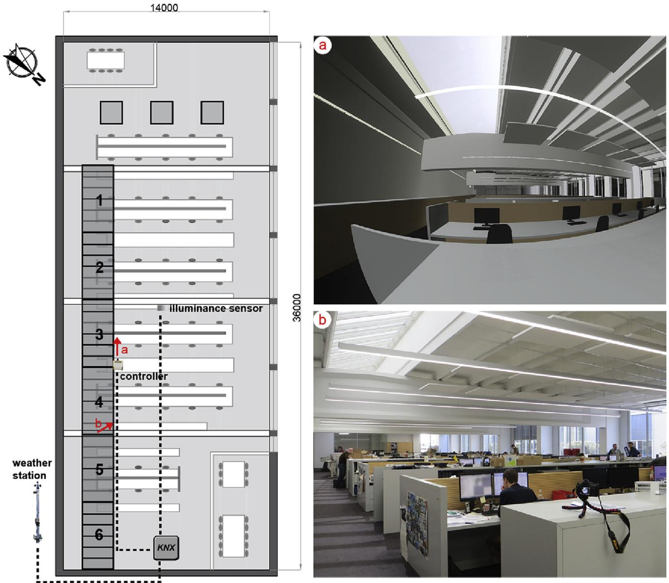
Fig. 4. Plan view of the open office space (left) with the indicated position of the illuminance sensor, the controller system, the blinds (1–6) and the weather station. Two images (right) show the view direction of the controller system (a) and another position in the room (b).
