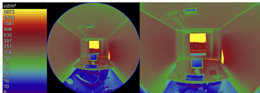
Fig. 1. The difference between a luminance map of the high-resolution camera (left) and the low-resolution camera (right).
