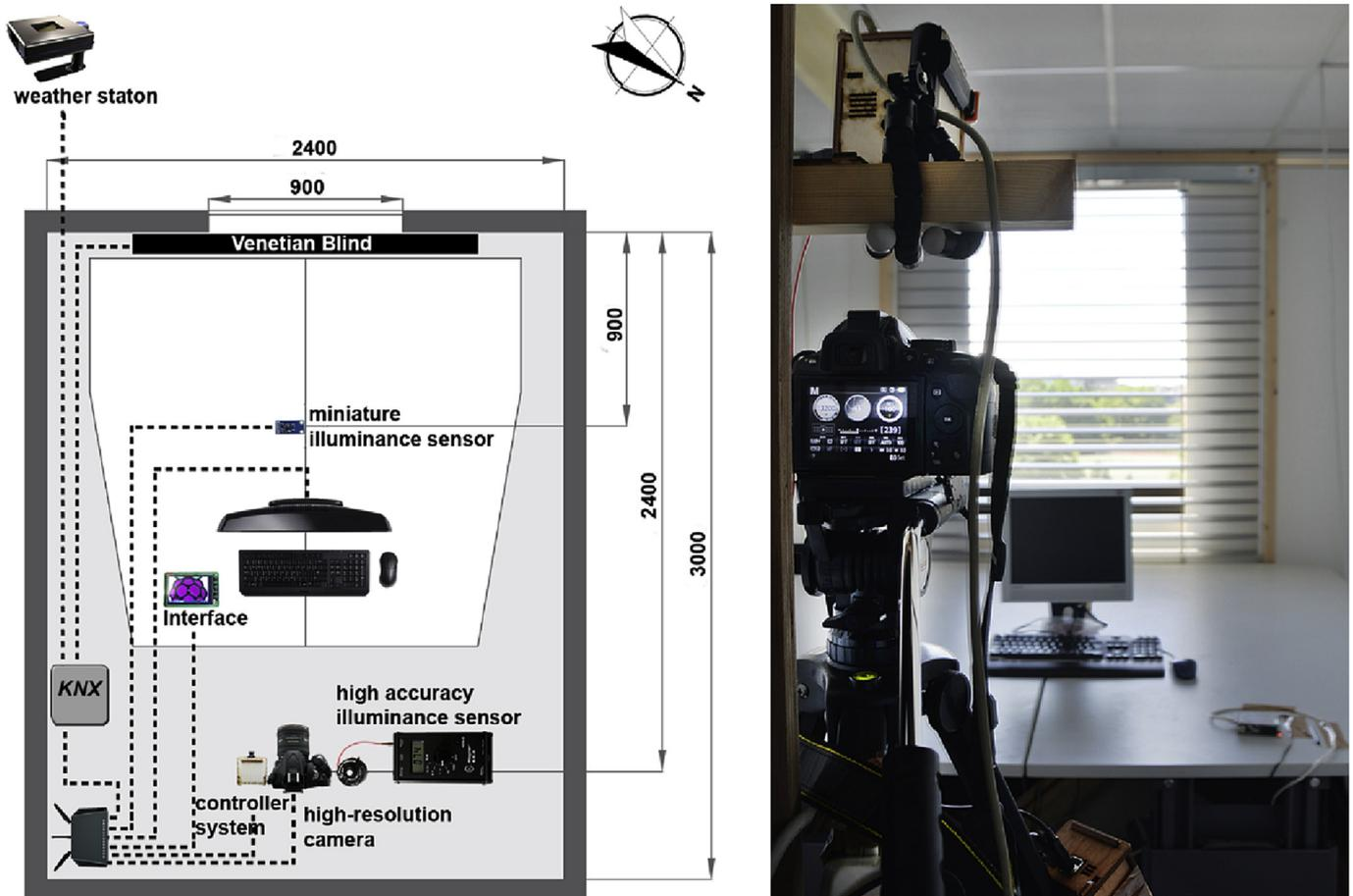
**Fig. 3.** Plan view of mock-up office room (left) and the position of the high-resolution camera, the controller system and the illuminance sensors in the office room (right). All dimensions are shown in millimetres.
