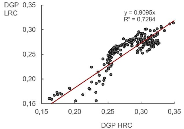
Fig. 2. The comparison of the calculated DGP value of the calibrated high-resolution camera (HRC) and the low-resolution camera (LRC) shows that the DGP of the LRC is underestimated.
