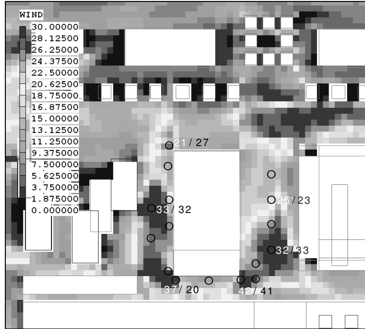
Figure 3: Comparison between the results of wind tunnel data and CFD for the second model in probability of exceedance P(V_{loc} > 5 \text{ m/s}) . White numbers CFD results, black numbers wind tunnel results.
