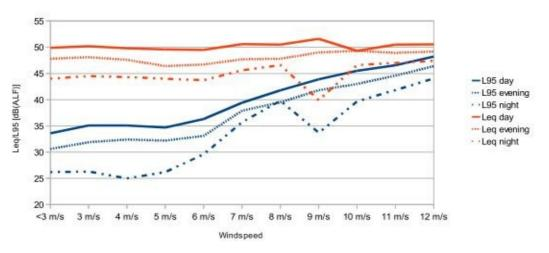
Figure 5 – Measured  $L_{95}$  and  $L_{eq}$  in dB(A,LF) plotted against wind-speed
